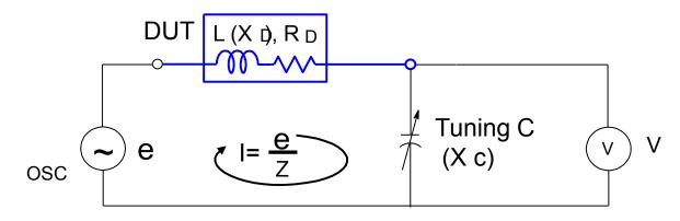
$$X_{C} = \frac{V}{I} = \frac{R_{D}V}{e} \text{ (at resonance)}$$
