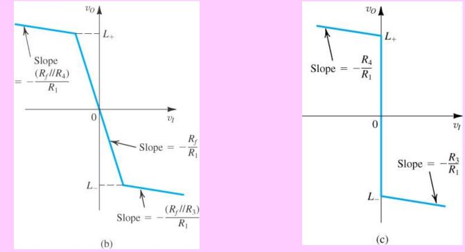
≻Transfer characteristic of the limiter circuit;
