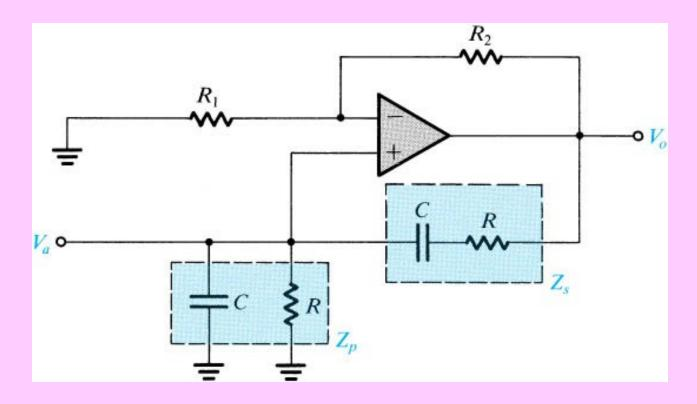
A Wien-bridge oscillator without amplitude stabilization.
