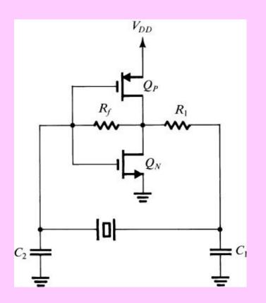
A Pierce crystal oscillator utilizing a CMOS inverter as an amplifier.
