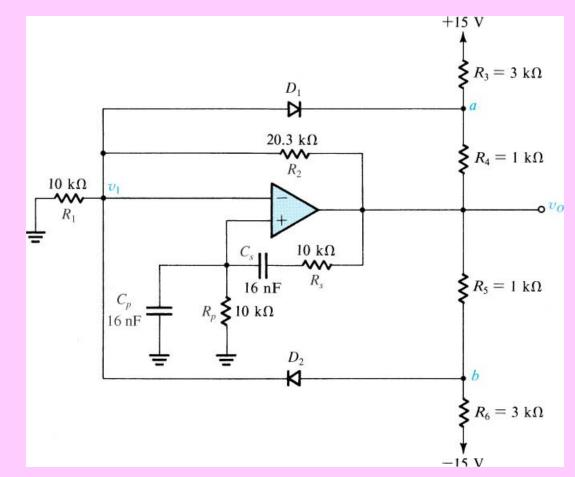
A Wien-bridge oscillator with a limiter used for amplitude control.
