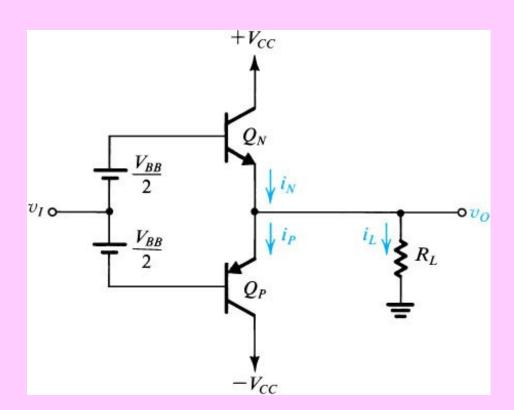
A bias voltage  $V_{BB}$  is applied between the bases of  $Q_N$  and  $Q_P$ , giving rise to a bias current  $I_Q$ . Thus, for small  $V_I$ , both transistors conduct and crossover distortion is almost completely eliminated.
