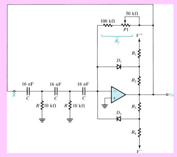
A practical phase-shift oscillator with a limiter for amplitude stabilization.
