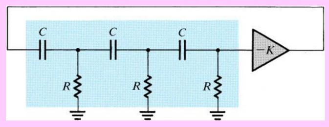
The circuit consists of a negative-gain amplifier and three-section RC ladder network.
