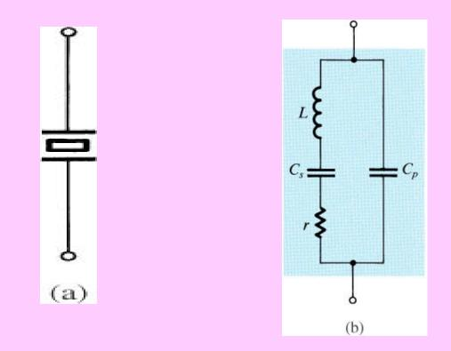
A piezoelectric crystal. (a) Circuit symbol. (b) Equivalent circuit.
