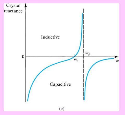
Crystal reactance versus frequency (neglecting the small resistance r, ).
