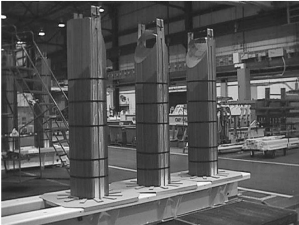
5 "E"-assembly, prior to addition of coils and insertion of top yoke.
