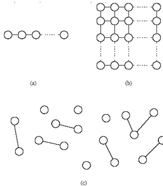
Examples of sparse graphs: (a) a linear graph, in which each vertex has two incident edges; (b) a grid graph, in which each vertex has four incident vertices; and (c) a random sparse graph.
