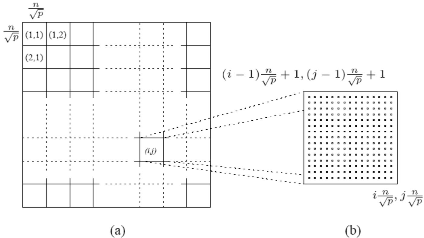
(a) Matrix  $D^{(k)}$  distributed by 2-D block mapping into  $\sqrt{p} \times \sqrt{p}$  subblocks, and (b) the subblock of  $D^{(k)}$  assigned to process  $P_{i,j}$ .
