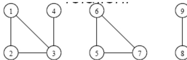
A graph with three connected components:  $\{1,2,3,4\}$ ,  $\{5,6,7\}$ , and  $\{8,9\}$ .
