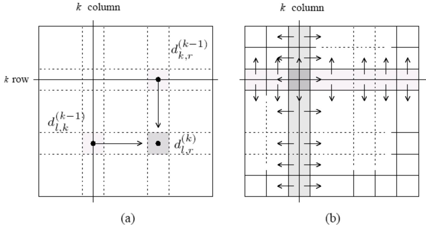
(a) Communication patterns used in the 2-D block mapping. When computing  $d_{i,j}^{(k)}$ , information must be sent to the highlighted process from two other processes along the same row and column. (b) The row and column of  $\sqrt{p}$  processes that contain the  $k^{\text{th}}$  row and column send them along process columns and rows.
