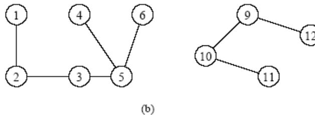
Part (b) is a depth-first forest obtained from depth-first traversal of the graph in part (a). Each of these trees is a connected component of the graph in part (a).
