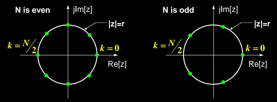
If N is even, the filter has a pair of real-valued poles  $z = \pm r$
