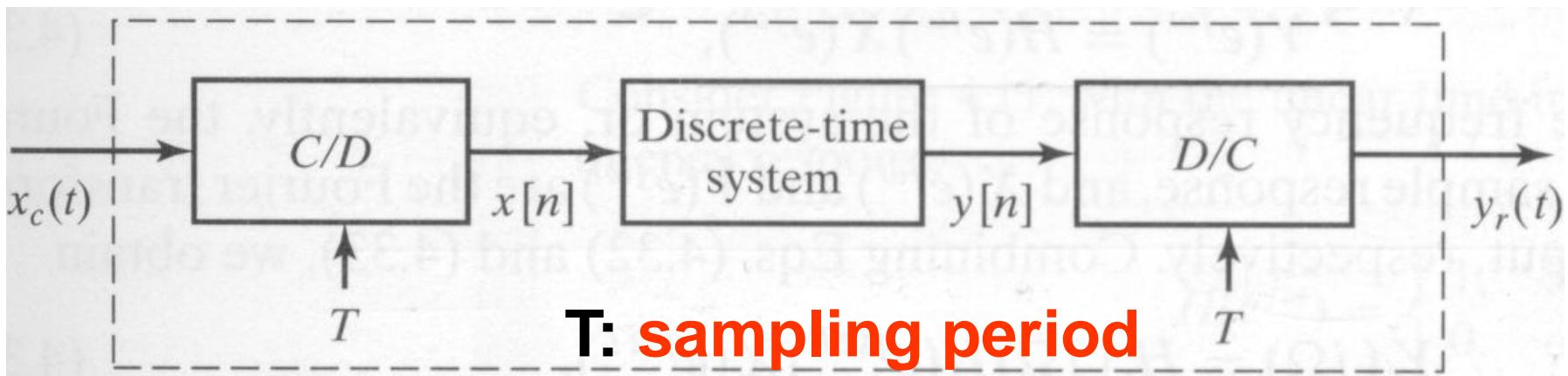
$$x[n] = x_c(nT), \quad f=1/T: \text{sampling frequency}$$
