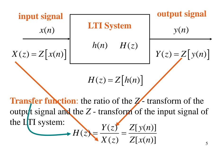
LTI system: the Z-transform of the constant coefficient linear difference equation under zero initial conditions:
