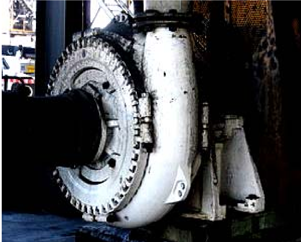
Figure of Centrifugal Pump
