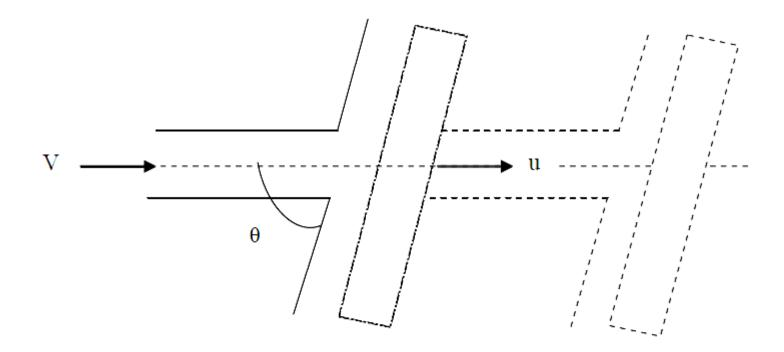
Force exerted by jet on the inclined plate in the direction normal to the jet
