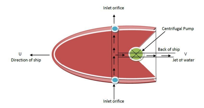
Force exerted by the jet on the ship = mass of water issuing/s x change in velocity
