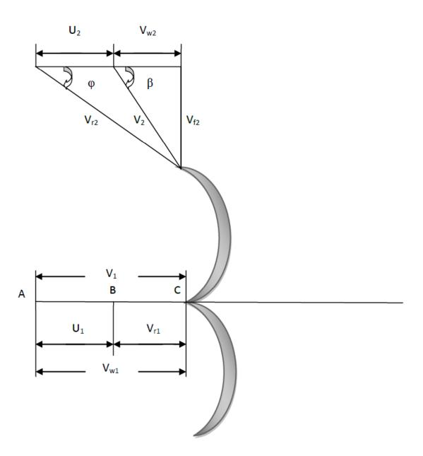
The velocity  $\Delta$  at inlet will be a straight line,
