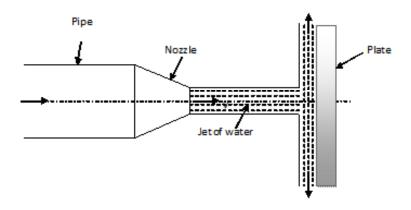
V = velocity of jet, d = diameter of the jet, a = area of x - section of the jet
