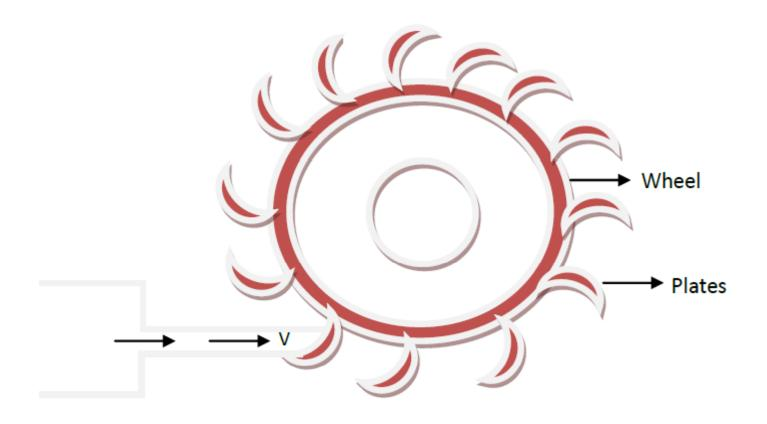
Force exerted by the jet on the plate in the direction of motion of plate = Mass/sec x (Initial velocity - Final velocity)  $F_{v} = \rho aV (V - u)$
