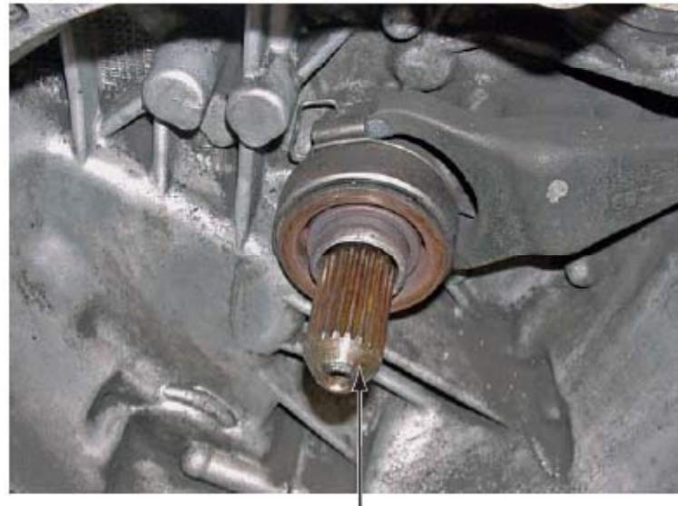
Figure 69.16 This front-wheel-drive transaxle does not use a pilot bearing.
