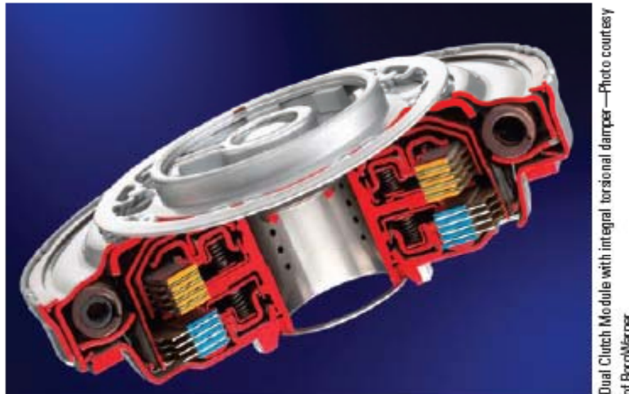
Figure 69.23 A dual clutch transmission employs two clutches that alternately connect engine output to transmission input shafts for odd-numbered gears or even-numbered gears, respectively.
