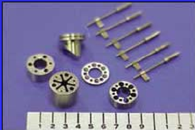
Small parts made using EDM
