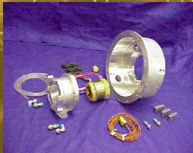
Motor/Generator, transfers energy to and from the rotor
