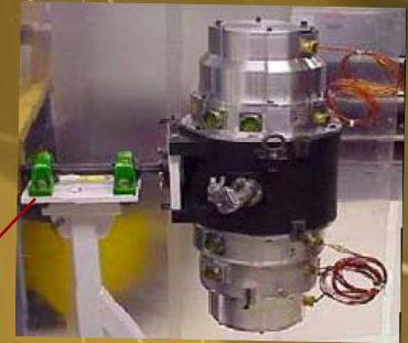
Housing, A structure used to hold the stationary components together. Can also act as a vacuum chamber
