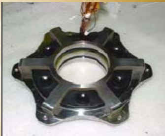
Magnetic Bearing, used to levitate rotor. These non-contact bearings provided low loss, high speeds, and long life
