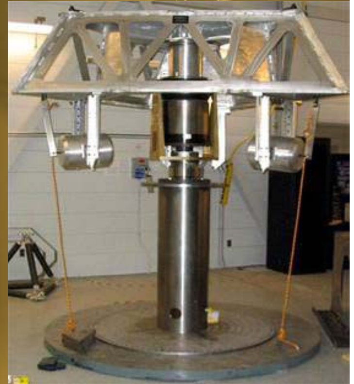
A completed mini-Agile Multi-Purpose Satellite Simulator is shown with three flywheel mass simulators that spin between 16,000 and 40,000 revolutions per minute.
