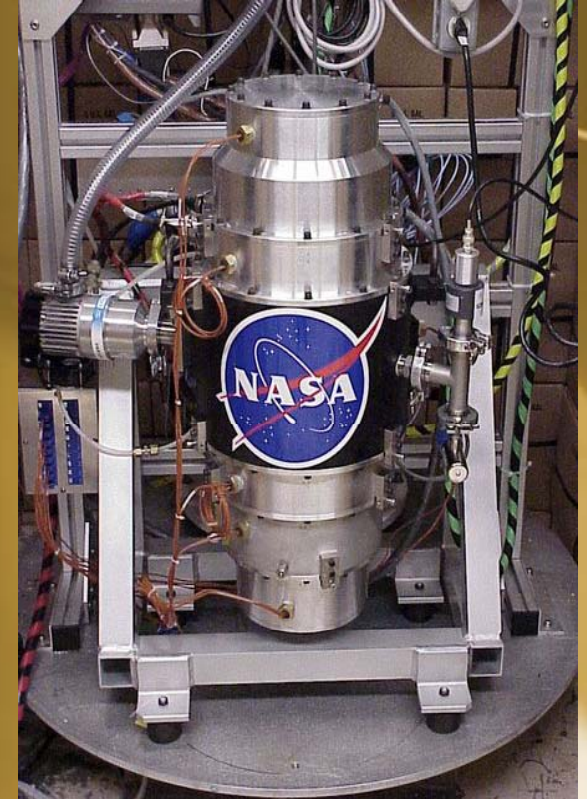
NASA G2 Flywheel Module - The Glenn Flywheel Development Team designed, built and successfully operated the new G2 flywheel to 41,000 RPM on September 2nd, 2004
