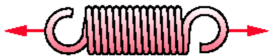
(b) Helical extension springs. Pull —wide load and deflection range—round or rectangular wire, constant rate.
