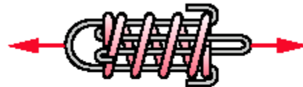
(c) Drawbar springs. Pull —uses compression spring and drawbars to provide extension pull with fail-safe, positive stop.
