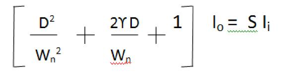
Example – -Piezoelectric pickup -Spring mass system -Pen control system on X-Y plotters -U-V Galvanometer
