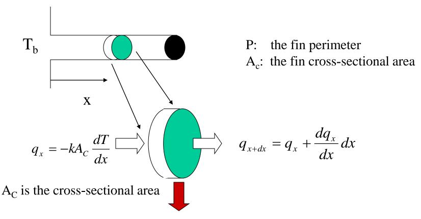
$dq_{conv} = h(dA_S)(T - T_{\infty})$ , where  $dA_S$  is the surface area of the element
