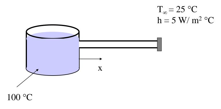
We can model the pot handle as an extended surface. Assume that there is no heat transfer at the free end of the handle. The condition matches that specified in the fins Table, case B. h=5 W/ m<sup>2</sup> °C, P=2W+2t=2(0.03+0.005)=0.07(m), k=237 W/m °C, A<sub>C</sub>=Wt=0.00015(m<sup>2</sup>), L=0.2(m) Therefore,  $m=(hP/kA_C)^{1/2}=3.138$ ,  $M=\sqrt{(hPkA_C)(T_b-T_{\infty})}=0.111\theta_b=0.111(100-25)=8.325(W)$
