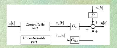
Figure 17.1: Controllable-uncontrollable decomposition
