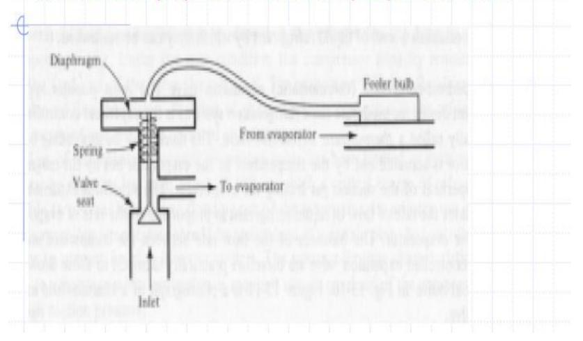
Feeler bulb is filled with same refrigerant as in system and is clamped to the outlet of the evaporator. If too little refrigerant is in the evaporator, it will be very superheated at the exit. This will make the refrigerant in the feeler bulb evaporate, increasing the pressure on the diaphragm. This will open the valve further, letting more refrigerant in, decreasing the temperature at the evaporator exit.
