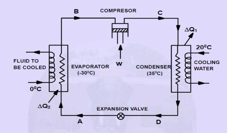
Fig.6.5. Simple vapour compression system
