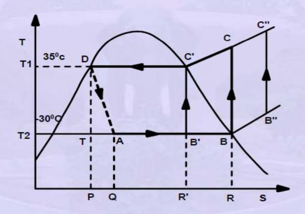
Fig.6.5.1. T-s diagram of refrigeration cycle
