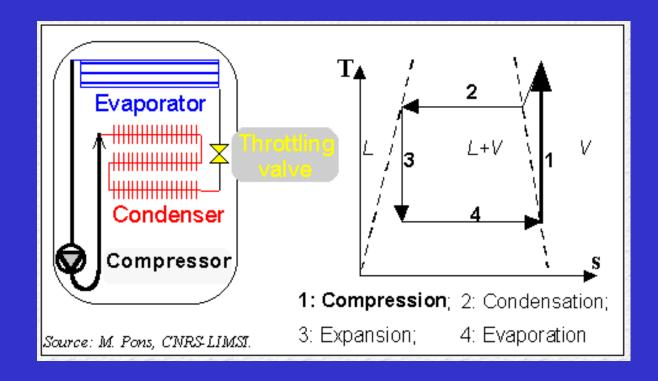
Vapor is compressed and its temperature increases
