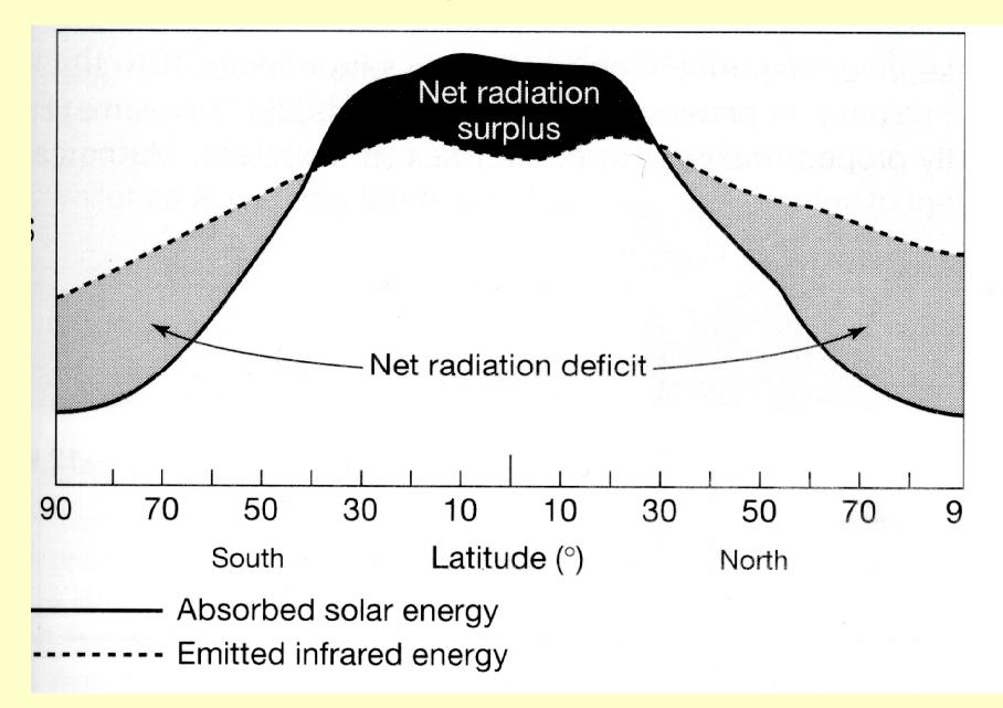
Radiation is not evenly distributed over the Surface of the earth. The northern latitudes have an energy deficit and the low latitude/ equator has an excess. But the low latitudes don't indefinitely get hotter and the northern latitudes don't get colder.
