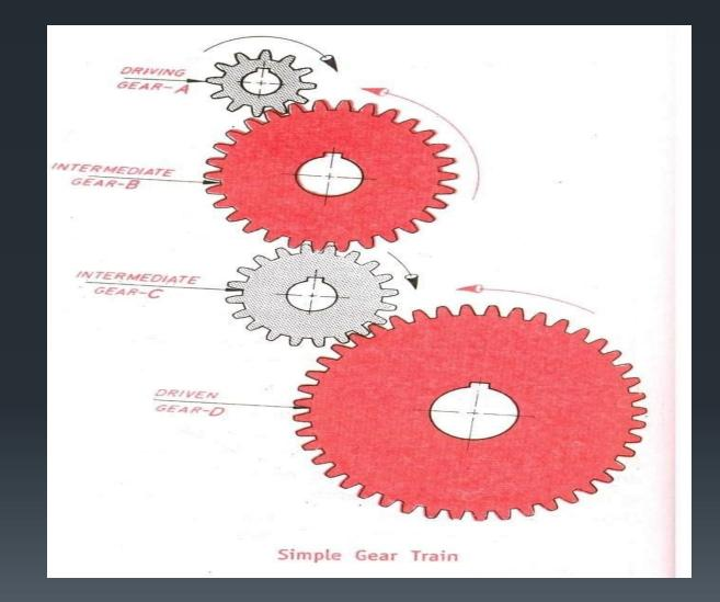
The velocity ratio of the gear train showr is obtained by multiplying
