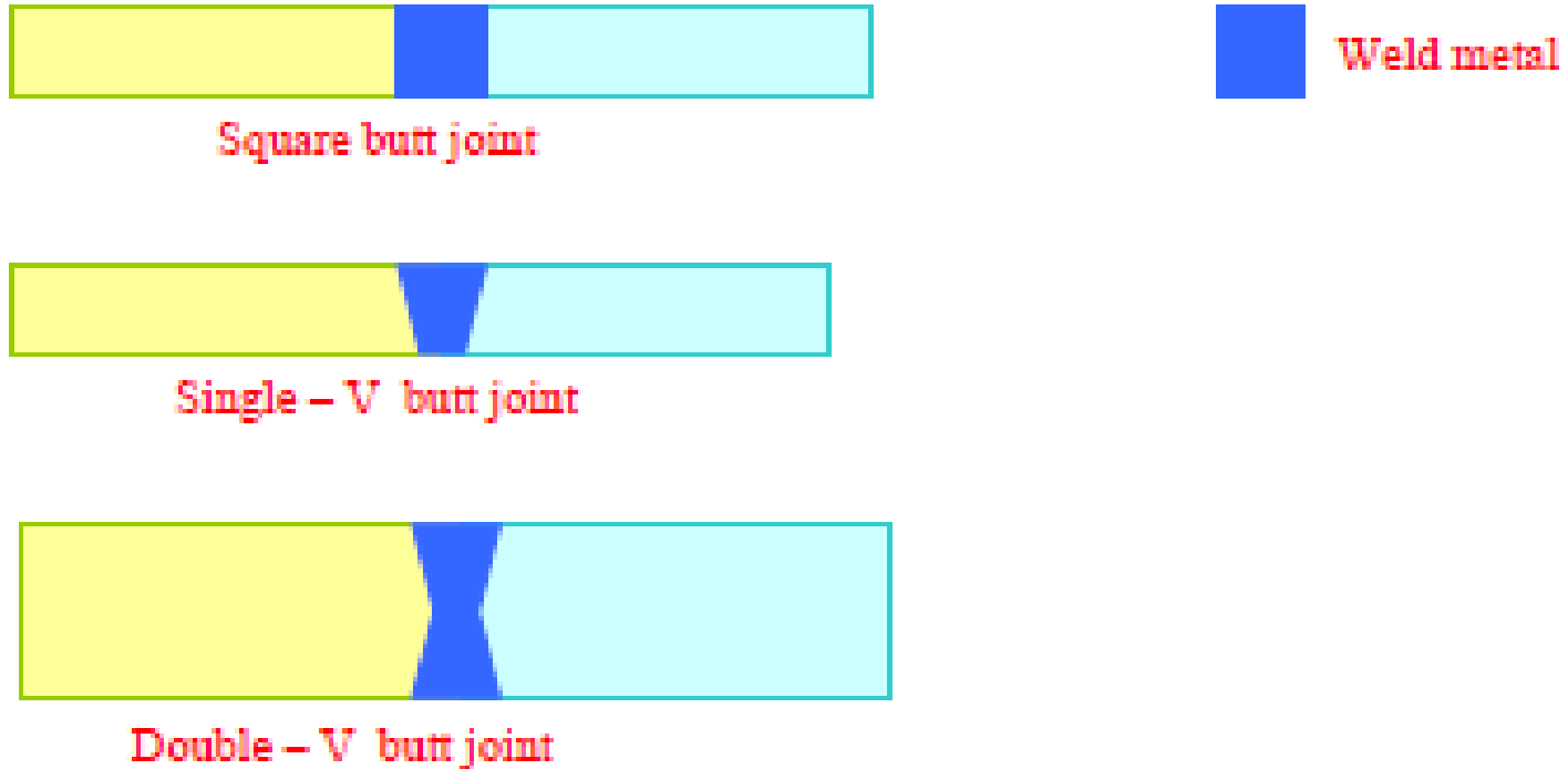
Figure 10.3.2: Different types of butt joints
