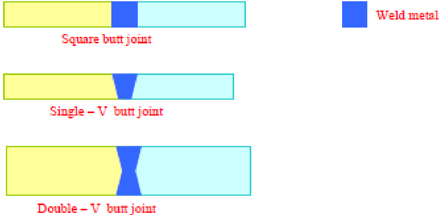
Figure 10.3.2: Different types of butt joints
