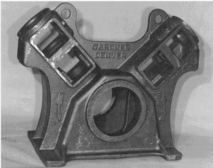
Figure 11.1 A large sand casting weighing over 680 kg (1500 lb) for an air compressor frame (photo courtesy of Elkhart Foundry).
