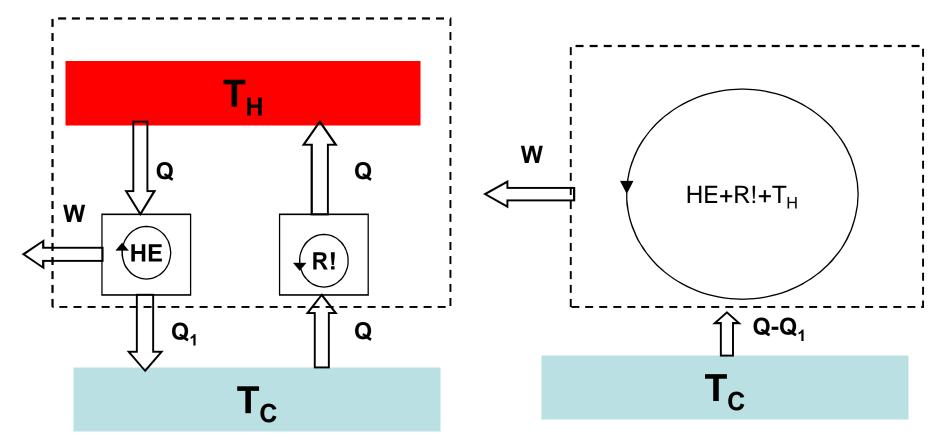
KP statement requires the device in contact with the single reservoir (here at  $T_c$ ) to be a cyclic device. Because nothing happens to the  $T_H$  reservoir ( $Q_{in}=Q_{out}=Q$ ). the combined device (HE+R!+T<sub>H</sub>) is a cyclic device.
