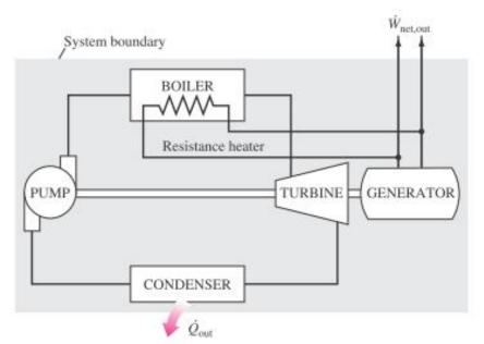
**Not OK!** Produces net energy output  $(\dot{Q}_{out} + \dot{W}_{out})$ without energy input.
