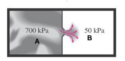
A membrane separates a gas in chamber A from vacuum in chamber B. The membrane is ruptured and the gas expands Into chamber B until pressure equilibrium is established. The process is so fast and the container is insulated enough such that negligible heat transfer takes place between the gas and the surroundings during this process.
