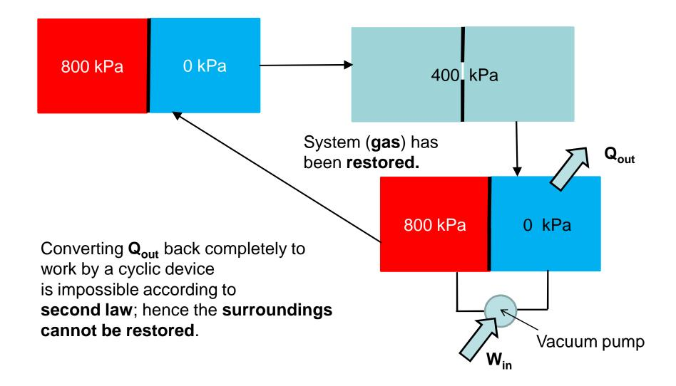
Another method to show that unrestrained expansion is an irreversible process: constructing a PMM2 that uses the reversed process.
