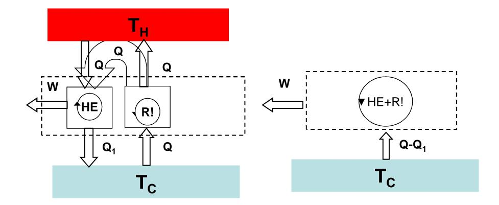
T<sub>H</sub> can be eliminated and Q can be fed directly to H from R
