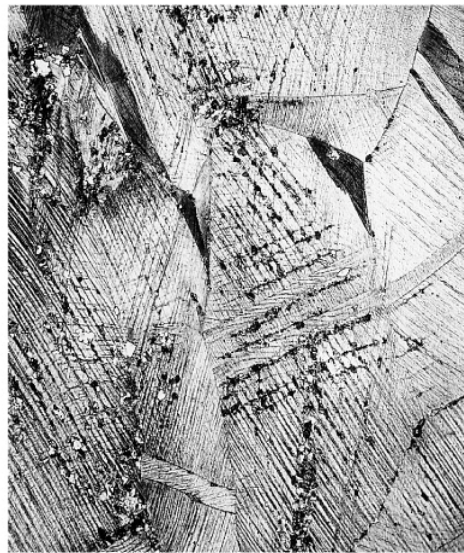
Initial recrystallization; After 3 seconds, 580°C
