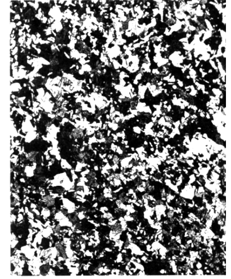
Complete recryst. after 8 seconds
