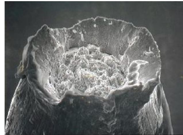
“cup and cone” fracture
