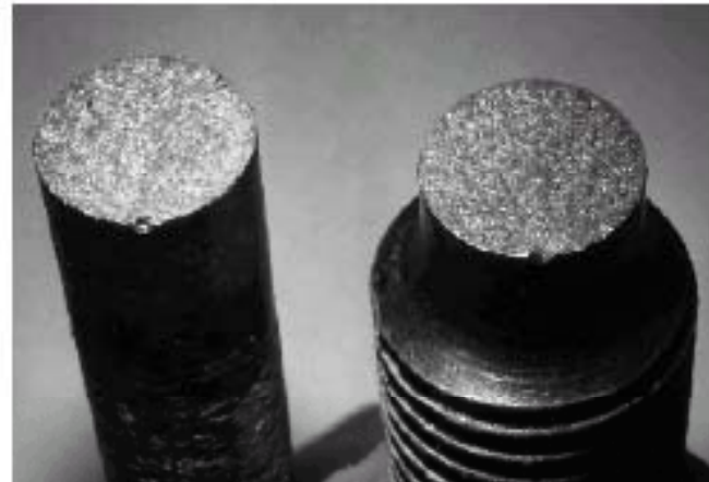
Brittle fracture in a mild steel
