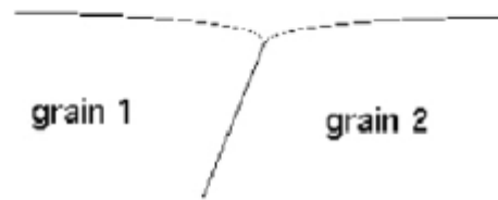
Fig. 3(b): Polished sample held at austenitisation temperature. Grooves develop at the prior austenite grain boundaries due to the balancing of surface tensions at grain junctions with the free surface. Micrograph courtesy of Saurabh Chatterjee .
