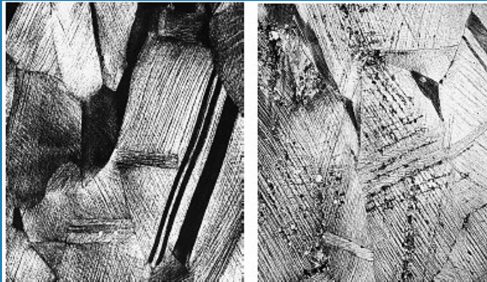
FIGURE 7.21 Photomicrographs showing several stages of the recrystallization and grain growth of brass. (a) Cold-worked (33%CW) grain structure. (b) Initial stage of recrystallization after heating 3 s at 580°C (1075°F); the very small grains are those that have recrystallized. (c) Partial replacement of cold-worked grains by recrystallized ones (4 s at 580°C). (d) Complete recrystallization (8 s at 580°C). (e) Grain growth after 15 min at 580°C. (f) Grain growth after 10 min at 700°C (1290°F). All photomicrographs 75 \times . (Photomicrographs courtesy of J. E. Burke, General Electric Company.)
