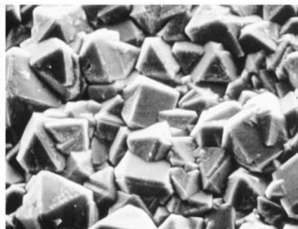
FIGURE 12.16 Scanning electron micrograph of a diamond thin film in which is shown numerous multifaceted microcrystals. 1000 \times . (Photograph courtesy of the Norton Company.)
