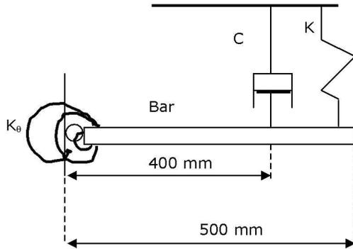
77. The un-damped natural frequency of oscillations of the bar about the hinge point is
