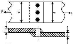
Width of the plate w=200 mm, thickness of the plate t=5 mm, number of rivets n=3, diameter of the rivet  $d_r = 10$ mm, diameter of the rivet hole  $d_h = 11$ mm, allowable tensile stress of the plate  $\sigma_P = 200MPa$ , allowable shear stress of the rivet  $\sigma_s$  = 100 MPa and allowable bearing stress of the  $\sigma_c$  = 150 MPa
