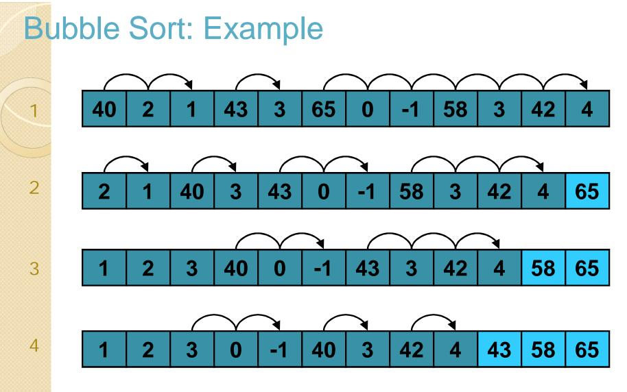
Notice that at least one element will be in the correct position each iteration.
