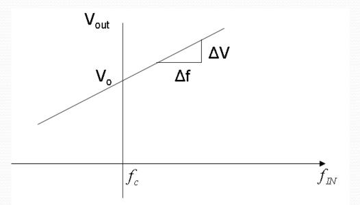
We define  $V_o$  as the output when  $f_{IN} = f_c$ , the nominal input frequency.
