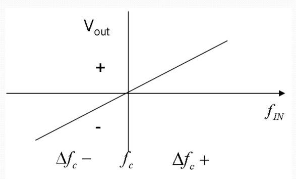
The important point is that  $V_{OUT} = K\alpha V_{IN}$ . If  $V_{IN} = m(t)$  then the output contains the message signal m(t), and the FM signal has been demodulated.
