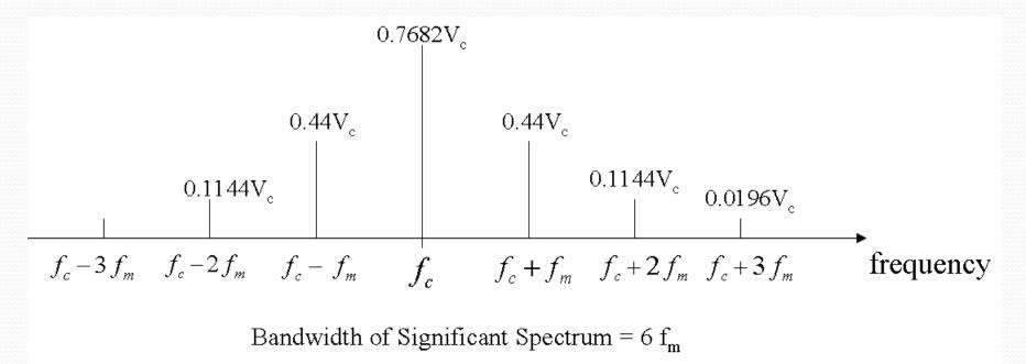
As shown, the bandwidth of the spectrum containing significant components is  $6f_m$ , for  $\beta = 1$ .
