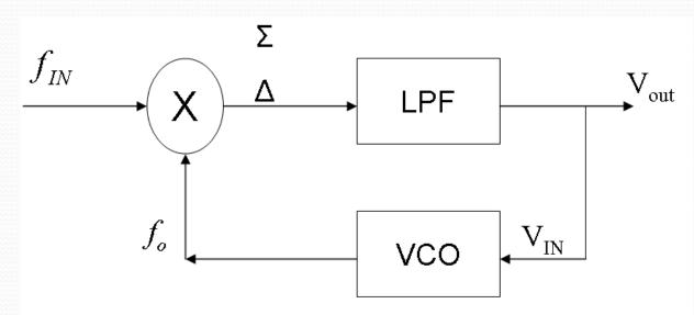
Note the similarity with a synchronous demodulator. The loop comprises a multiplier, a low pass filter and VCO (V/F converter as used in a frequency modulator).
