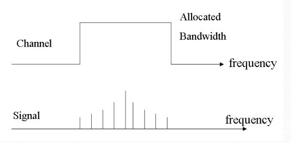
However, many signals (*e.g.* FM, square waves, digital signals) contain an infinite number of components. If we transfer such a signal via a limited channel bandwidth, we will lose some of the components and the output signal will be distorted. If we put an infinitely wide train through a tunnel, the train would come out distorted, the question is how much distortion can be tolerated?
