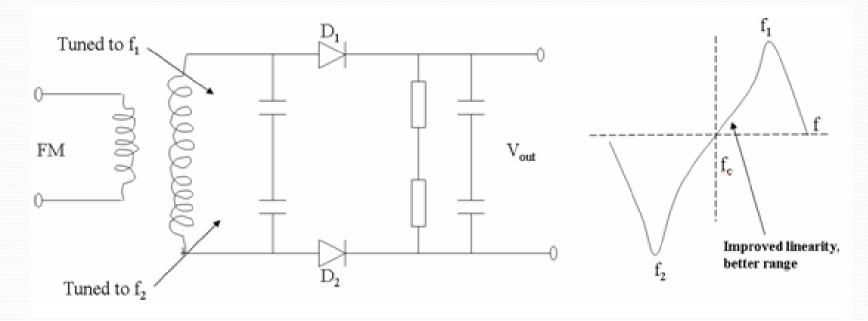
This gives the composite characteristics shown. Diode  $D_2$  effectively inverts the  $f_2$  tuned circuit response. This gives the characteristic 'S' type detector.
