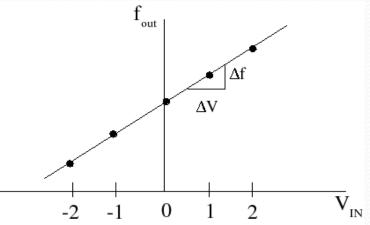
$f_c$ , the frequency output when the input is zero is called the undeviated or nominal carrier frequency.
