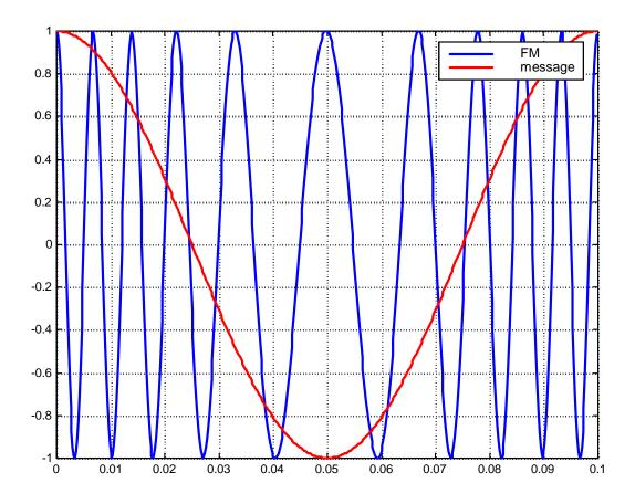
Inst.frequency Moves with the Message amplitude
