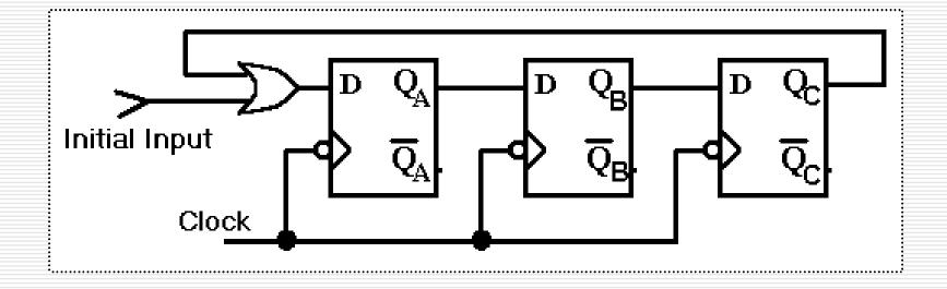
In Class: Build a ring counter using electronics simulation tools
