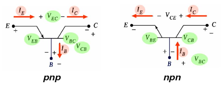
Two of the currents and two of the voltages are independent. If two of the currents or voltages are known, third terminal current or voltage is determined.
