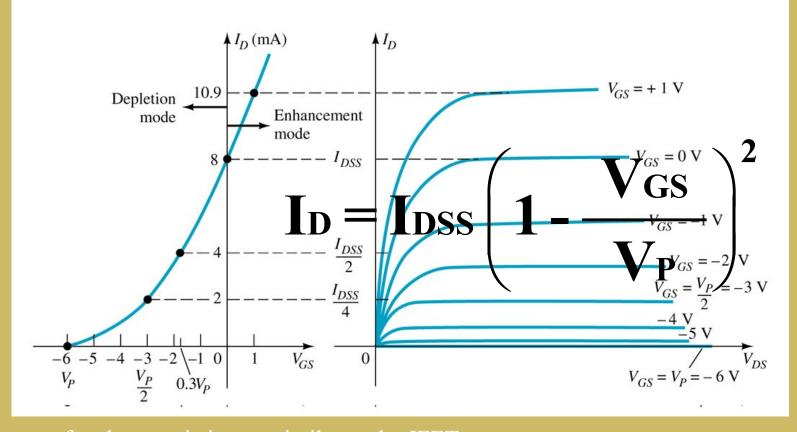
The transfer characteristics are similar to the JFET In Depletion Mode operation: When  $V_{GS} = 0V$ ,  $I_D = I_{DSS}$ When  $V_{GS} < 0V$ ,  $I_D < I_{DSS}$ When  $V_{GS} > 0V$ ,  $I_D > I_{DSS}$ The formula used to plot the Transfer Curve, is:
