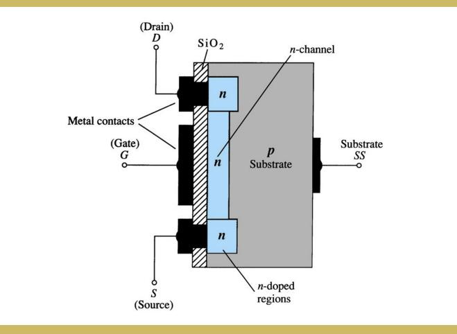
The Drain (D) and Source (S) leads connect to the to n-doped regions These N-doped regions are connected via an n-channel This n-channel is connected to the Gate (G) via a thin insulating layer of SiO<sub>2</sub> The n-doped material lies on a p-doped substrate that may have an additional terminal connection called SS
