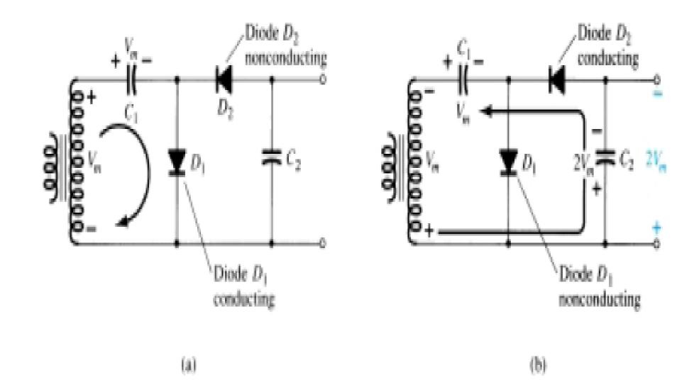
During the positive voltage half-cycle across the transformer, secondary diode D1 conducts (and diode D2 is cut off), charging capacitor C1 up to the peak rectified voltage (Vm). Diode D1 is ideally a short during this half-cycle, and the input voltage charges capacitor C1 to Vm.
