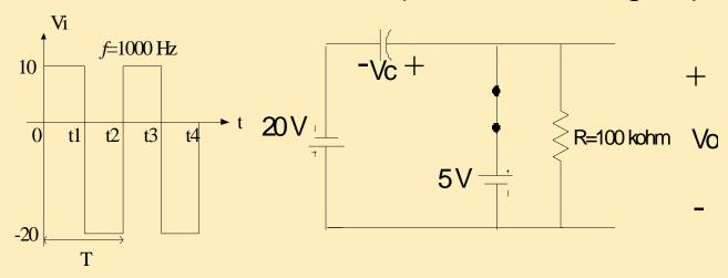
**Step 2:** During ON state assume capacitor will charge to a voltage level determined by the network. Find the store voltage capacitor & obtained Vo
