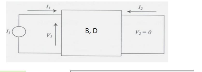
$$B = \frac{V_1}{-I_2} \quad | \quad V_2 = 0$$
