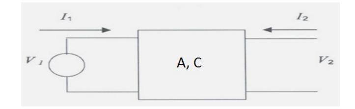
$$A = \frac{V_1}{V_2} \qquad | \quad |_2 = 0$$
