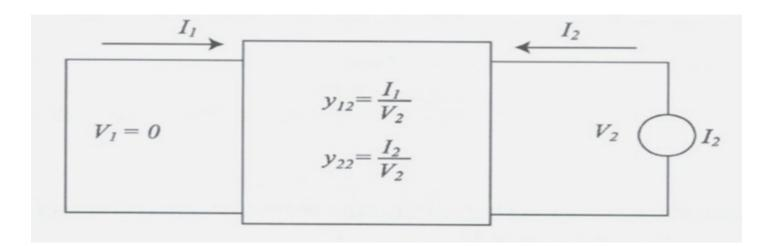
$$y_{12} = \frac{I_1}{V_2} |_{V_1} = 0$$
