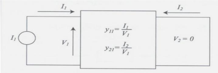
$$y_{11} = \frac{I_1}{V_1} |_{V_2} = 0$$
