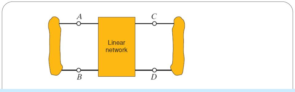
A two-port model is a description of a network that relates voltages a at two pairs of terminals
