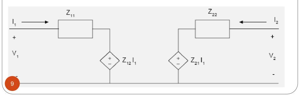
Case –I Assuming the output of the two port to be open circuit, I<sub>2</sub> =0
