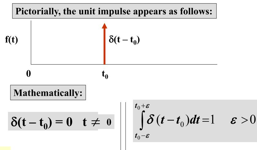
The Laplace transform of a unit impulse:
