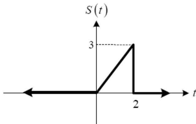
The signal between the interval of  $0 \leq t \leq 2$  is a line between two points  $P_1(t_1 = 0, s_1 = 0)$  and  $P_2(t_2 = 2, s_2 = 3)$  given by equation:
