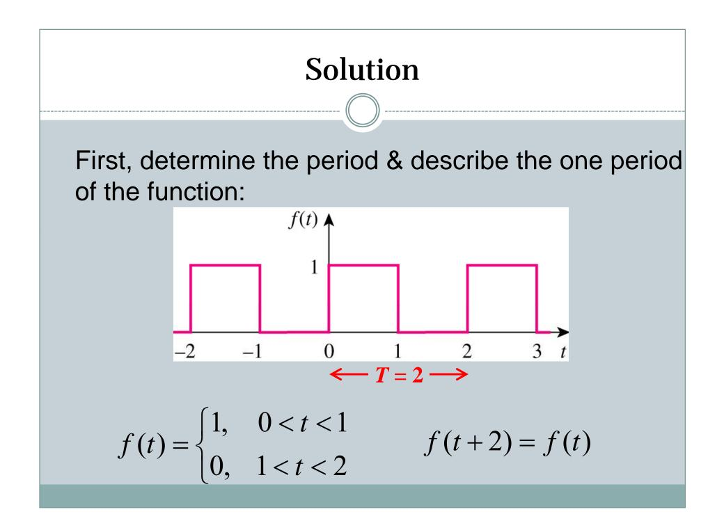
Then, obtain the coefficients  $a_0$ ,  $a_n$  and  $b_n$ :  $a_0 = \frac{2}{T} \int_0^t f(t) dt = \frac{2}{2} \int_0^2 f(t) dt = \int_0^1 1 dt + \int_0^2 0 dt = 1 - 0 = 1$ Or, since  $\int_{a}^{b} f(t)dt$  is the total area below graph y = f(t) over the interval [*a*,*b*], hence  $a_0 = \frac{2}{T} \int_0^T f(t) dt = \frac{2}{T} \times \begin{pmatrix} \text{Area below graph} \\ \text{over}[0,T] \end{pmatrix} = \frac{2}{2} \times (1 \times 1) = 1$
