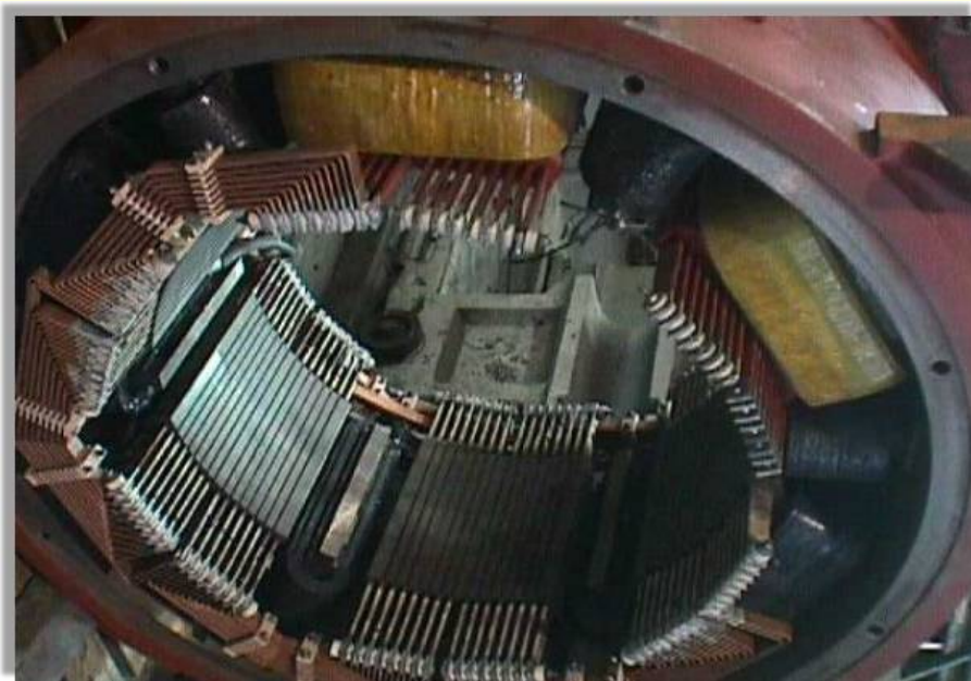
2000HP DC Motor field System
