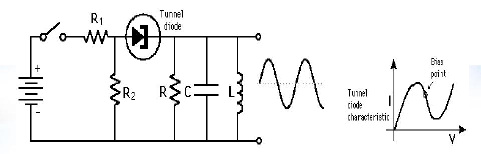
The <u>negative resistance region</u> of the tunnel diode makes oscillator action possible. The choice of network elements is designed to establish a load line such as shown in the fig. When the power is turned on, the terminal voltage of the supply will build up from 0V to a final value of E volts.
