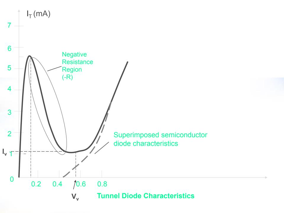
The peak current, I<sub>p</sub> of a tunnel diode can vary from a few microamperes to several hundred amperes. The peak voltage, however, is limited to about 600 mV. For this reason, a simple VOM with an internal dc battery potential of 1.5V can severely damaged a tunnel diode if applied improperly.
