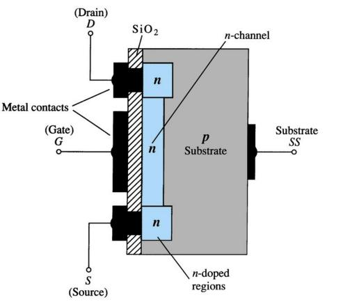
The Drain (D) and Source (S) leads connect to the to n-doped regions These N-doped regions are connected via an n-channel
