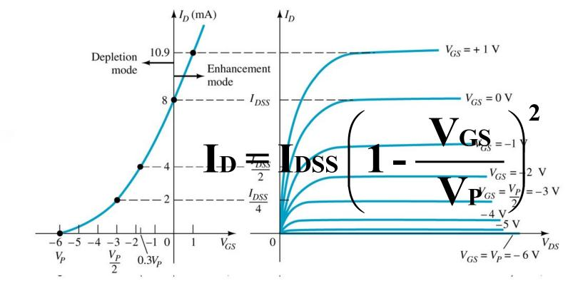
The transfer characteristics are similar to the JFET In Depletion Mode operation: When  $V_{GS} = 0V$ ,  $I_D = I_{DSS}$ When  $V_{GS} < 0V$ ,  $I_D < I_{DSS}$ When  $V_{GS} > 0V$ ,  $I_D > I_{DSS}$ The formula used to plot the Transfer Curve, is:
