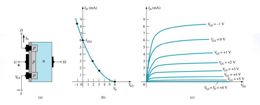
The p-channel Depletion mode MOSFET is similar to the n-channel except that the voltage polarities and current directions are reversed
