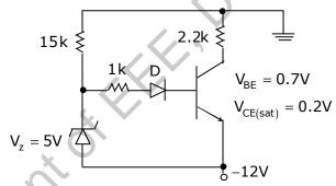
If the forward voltage drop of diode is 0.7V, then the current through collector will be  $% \left( {{\left[ {{{\rm{T}}_{\rm{T}}} \right]}_{\rm{T}}} \right)$
