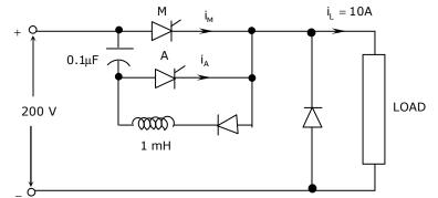
If the maximum value of load current is 10A, then the maximum current through the main (M) and auxiliary (A) thyristors will be
