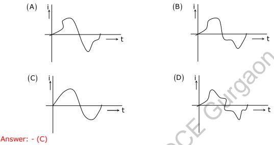
Exp: - It is an air core transformer. So, there is no saturation effect.
