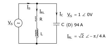
50. The power dissipated in the resistor R is
