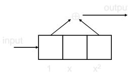
will multiply the input stream by  $x^2+1$  and the second shift register
